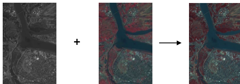
Figure 5. Image pan-sharpening with SPOT-4 images. (left) panchromatic image. (middle) multispectral image. (right) pansharpened image.
